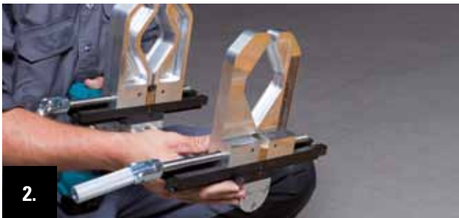
2. Adjust fitting slide in the front guide rail to the required pipe dimension and fix with locking bow.
