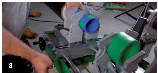
8. For adjustment of the welding depth press the calibration button in the middle of the machine frame up to the stop.
