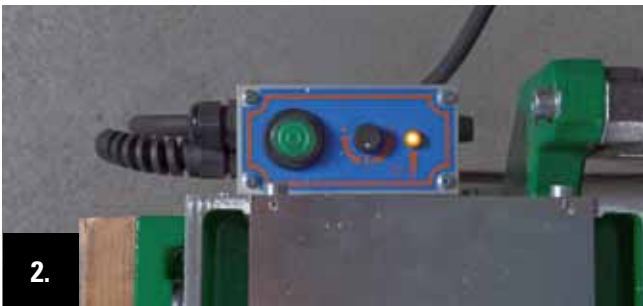
2. Plug the machine and check, if the yellow operation lamp is on.
