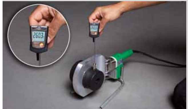
Measurement of temperature at the aquatherm- manual welding device (1400W )
