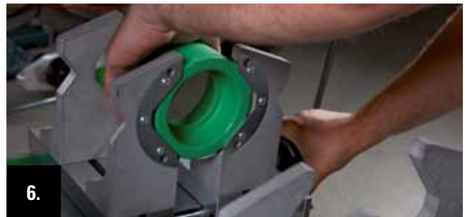
6. Fix the socket close to the stop und tighten the clamping jaws with the crank handle.
