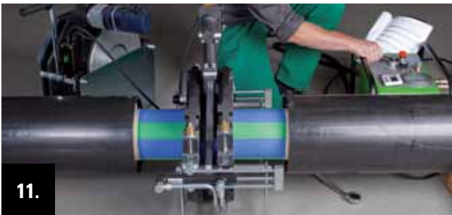
11. Drive the machine slide, by operating the hydraulic system, slowly against the welding plate. Then press the pipe ends until the predetermined adjustment pressure is achieved against the welding plate.
