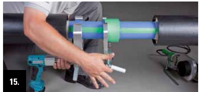
15. Release the clamping jaws on the fitting side by unscrewing the fixing jaw.
