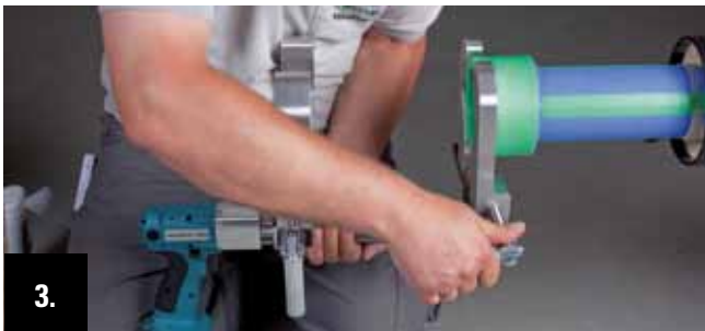
3. Push clamping jaws against the face side of the fitting up to the stop and tighten them with a fixing screw.
