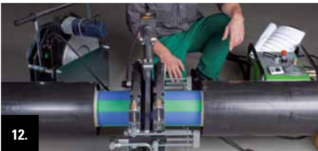
12. After the bead has achieved the preset height the pressure is reduced at the hydraulic system. Then the heating up phase starts. Now the face sides in which the face sides of the pipe ends are heated up to the required welding temperature.
